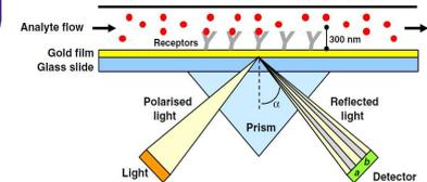
**Fig 5.** Principle of SPR experiment<sup>[8]</sup>. Protein of interest is immobilised on a sensor chip and potential ligands are flowed over the surface. Polarised light is directed to the chip, generating surface plasmons that absorb light at a critical angle. Refractive index varies proportionally to the amount of material bound on the surface.
